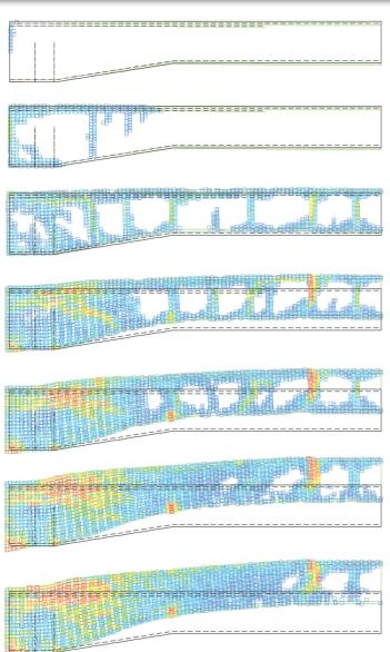
Structural nonlinear staged analysis of a gas explosion in a tunnel
